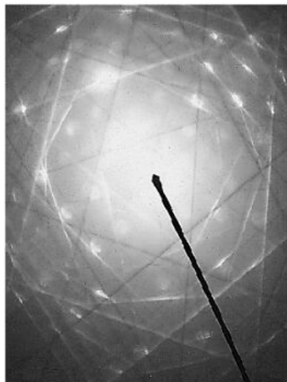
Transmission Kikuchi Pattern TEM, 250 kV
