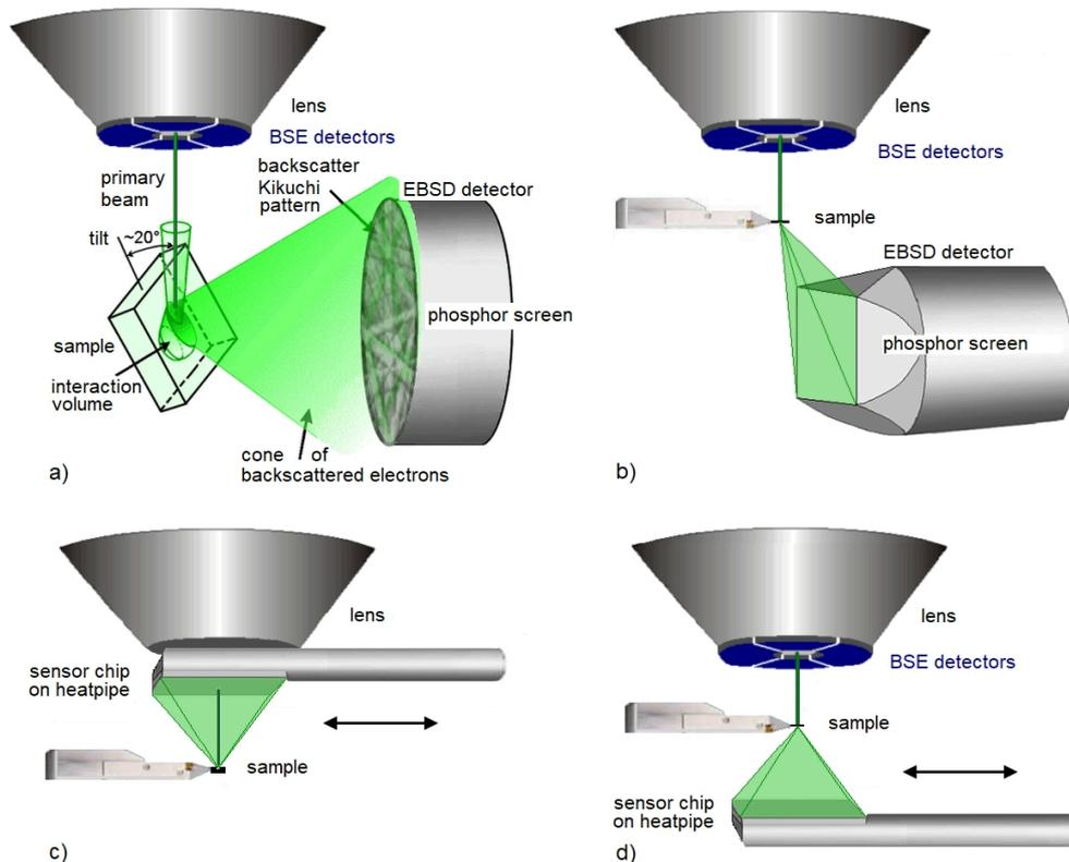
Figure 1 Kikuchi diffraction in the SEM. The conical sections of the recorded patterns are marked in green.
