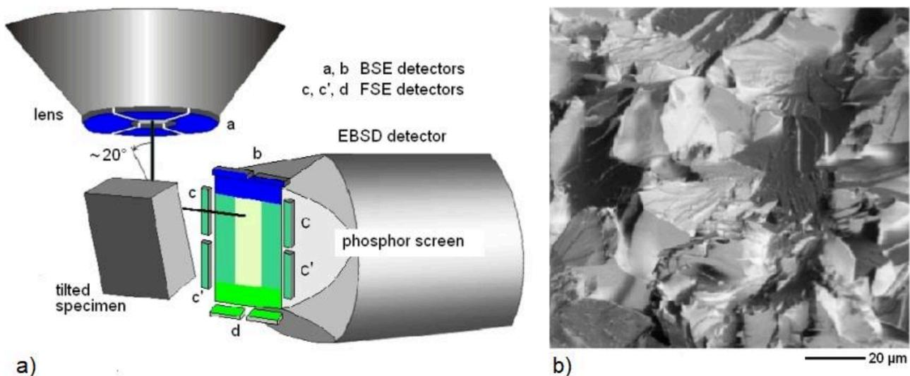
Figure 2 a) The conventional BKD detector used as a pixelated multi-area detector. Optional solid-state BSE (marked in blue) and FSE (marked in yellow) detectors are no longer required.
