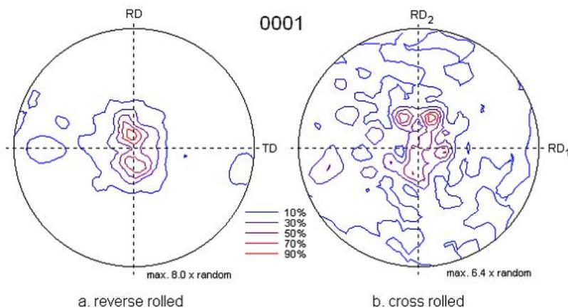
0001 pole-figures of a cross-rolled AM20 magnesium sheet.
