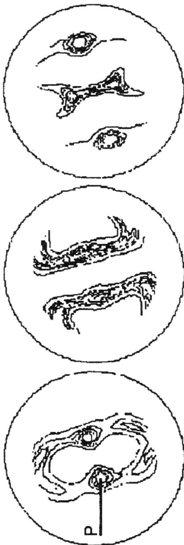
Figure 8: Pole figures acquired across the rivet bolt. The polar specimen direction  $P$  ( $\alpha = 35^\circ$ ,  $\beta = 83^\circ$ ) has been used for texture and residual strain mapping (cf. Figure 9).
