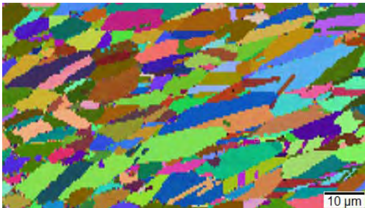
Figure 3: Crystal orientation maps of a Nickel specimen constructed from ACOM data.
